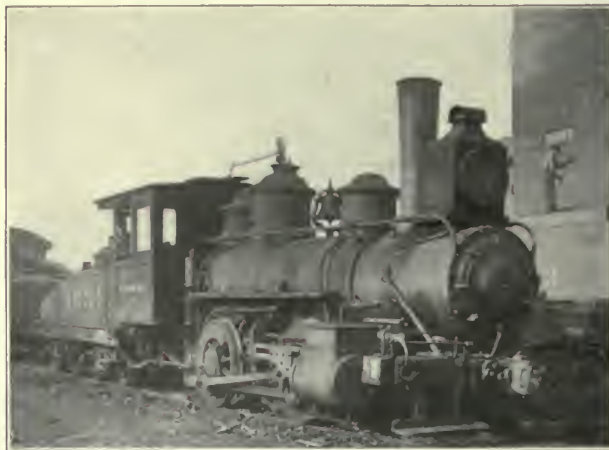
FIG. 390. LOCOMOTIVES. Switching Locomotive of the Four-wheel Type. This is a very light locomotive of the older type, used in switching service. At present it is engaged in light yard service. Chicago, Milwaukee & St. Paul Railway.
